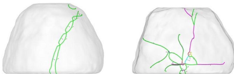
Figure : (left) dissociated dislocation introduced in Pt NP with a diameter of 20 nm. (Right) microstructure after a uniaxial compression of 8.6%.
